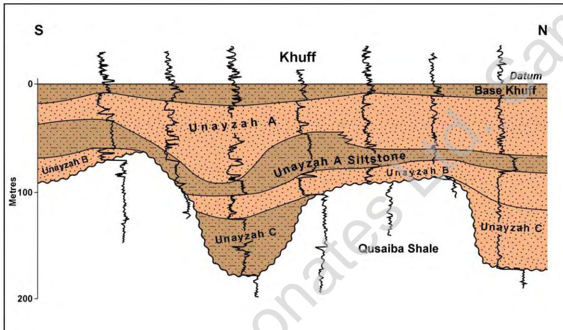
Figure 46 Correlation of Unayzah Formation sandbodies draping the pre Unayzah Unconformity. Cambridge Carbonates figure after Al Laboun (1986).
